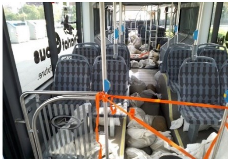
Figure 3. Loading the E-bus with sandbags
