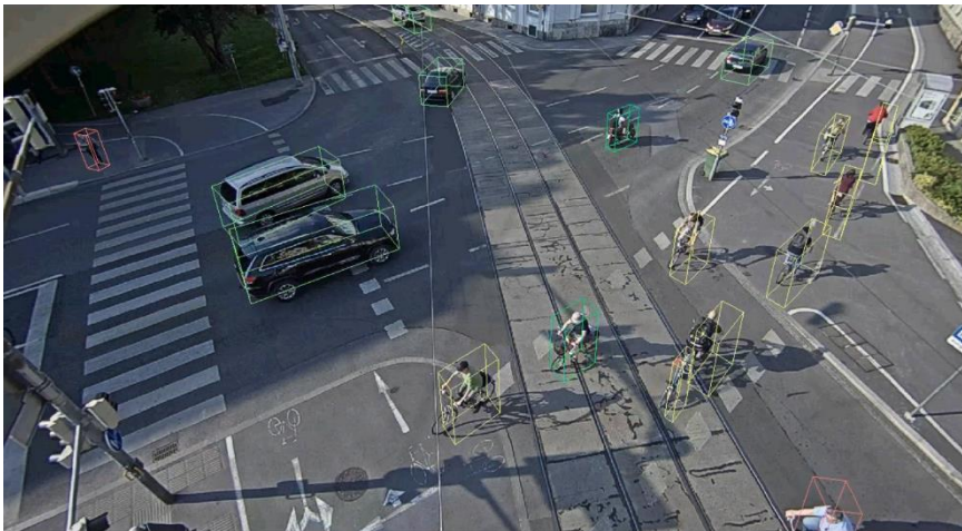
Figure 4. Results from the visual traffic analysis. The 3D-boxes show the position and type of the different road users.
