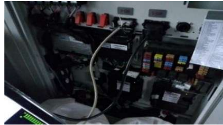
Figure 5. Connectors for S-CAN and V-CAN E-bus network
