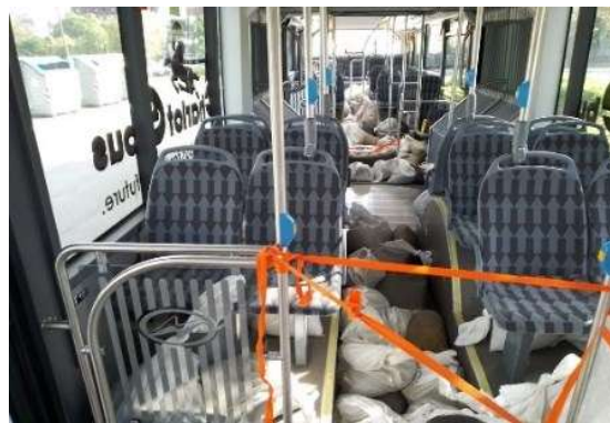
Figure 3. Loading the E-bus with sandbags
