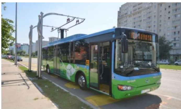
Figure 16. Electric Bus Higer A6L charging in Belgrade (source: Chariot Ltd)
