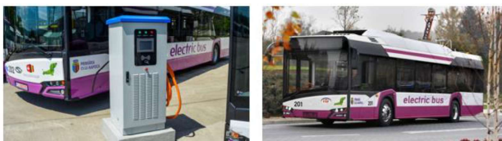
Figure 20. Charger stations: by cable (left) and by pantograf (right)
