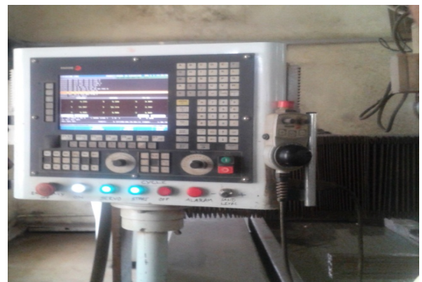
Fig. 5. Control Panel for Abrasive water jet Machine
