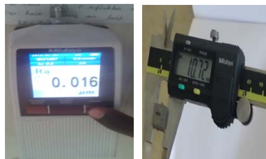
Fig. 7. (a) Surface Roughness measurent by using Talysurf (b) Kerf width is measeured y using Vernier Callipers.
