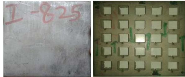
Fig. 2. Inconel Workpiece Before & After Machining
