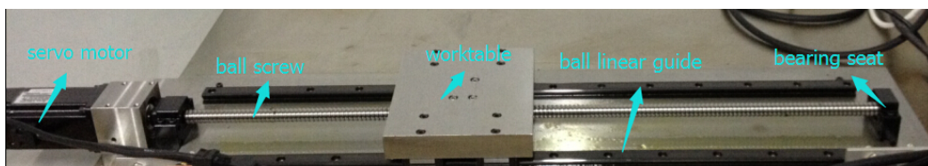
Figure 5. Feed drive system setup
