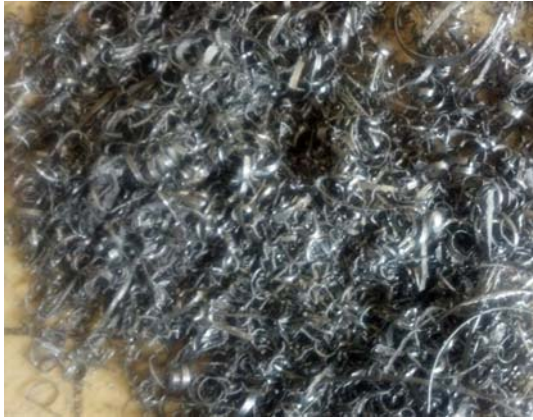
Fig. 5. Chip formed with the use of conventional cutting fluid
