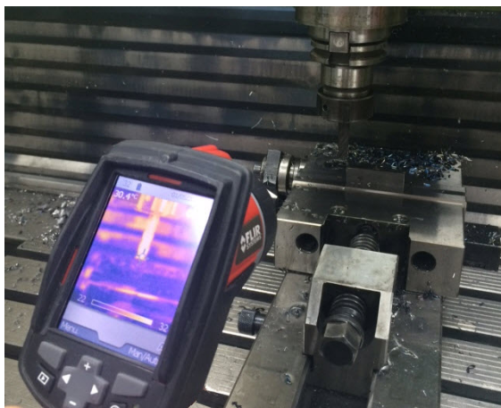
Fig. 1. Monitoring the temperature using infrared camera
