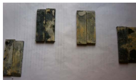
Fig. 2. Flux coated Ti6Al4V workpiece
