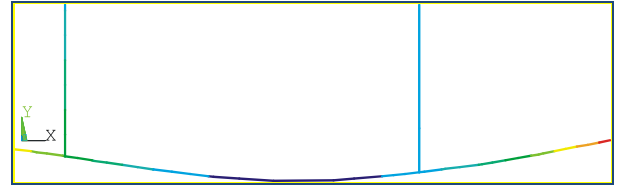
Fig. 6 Third natural frequencies of the test spindle
