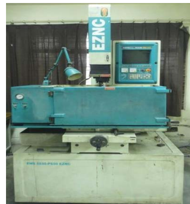
Fig.1. Physical set up of Electrical Discharge Machine
