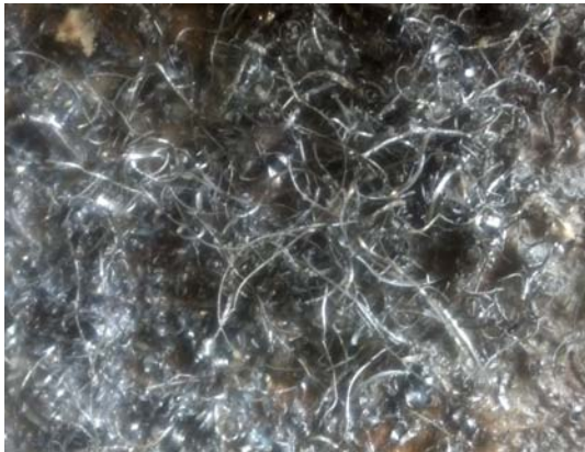
Fig. 6. Chip formed with the use of shea butter-based cutting fluid
