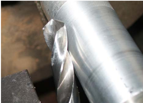
Fig. 10. Position of tool cutting edge against the workpiece
