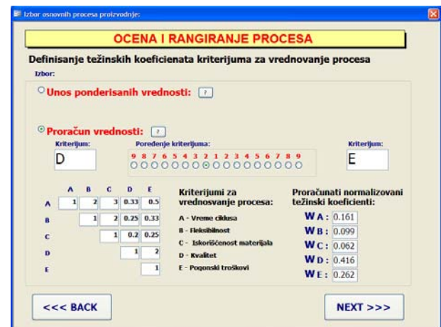
Fig. 6. Calculation of weight coefficients for evaluation of alternative solutions - Var1 - method (b)
