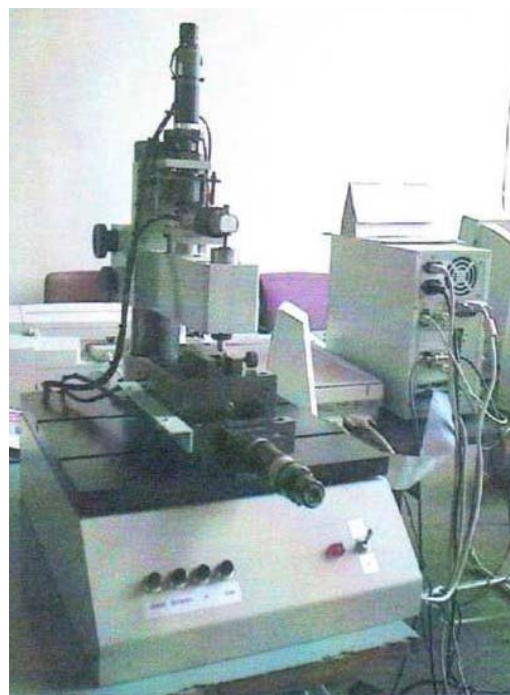
Fig.7 Scratch tester ST-99
