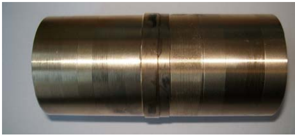
Fig. 13. View of an experimental workpiece, on the right – turning with a tool with rip radius, on the left – with a helical tool
