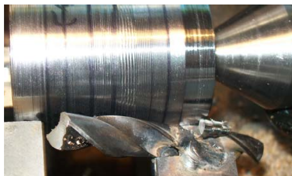
Fig. 4. View of machining process of turning titanium alloy
