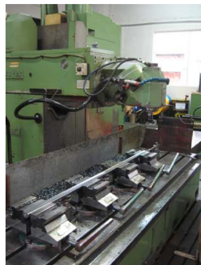
Fig. 1. Milling machine of the Zayer 3000 BF 3 type
