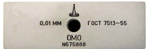
Fig. 2. General view of a stage object micrometer produced by LOMO (Russia) used in the tests
