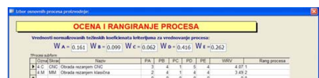
Fig.7. Results of evaluation and ranking of alternative processes for manufacturing the bearing ring - Var1
