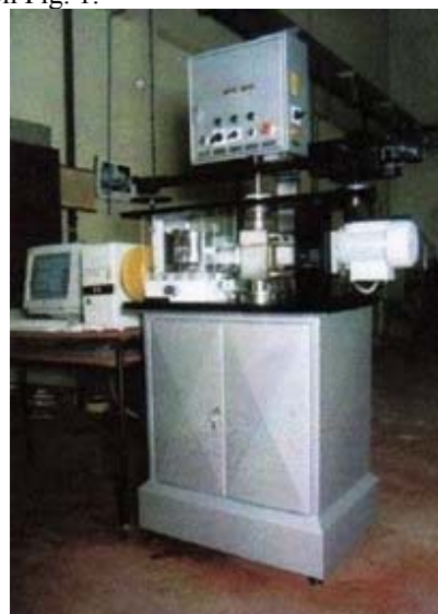
Fig.1 Tribometer "Block on Disk" TPD 2000
