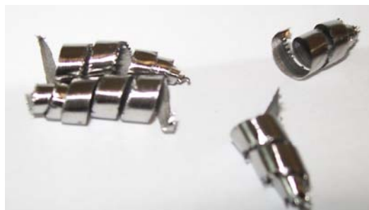
Fig. 5. Shape of chips obtained at turning titanium alloy with a helical tool
