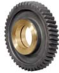
Fig. 6. Shows the timing gears for diesel engines made from austempered ductile iron EN-GJS-700-2 initial pearlite basis
