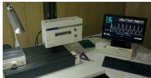
Figure 6. Device for the roughness measuring Taylor–Hobson, Form Talysurf
