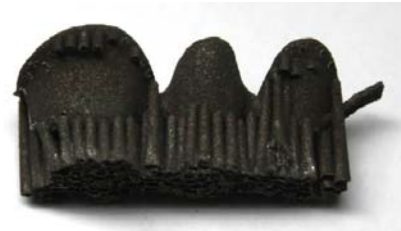
Fig. 10. SLM made construction with support structure
