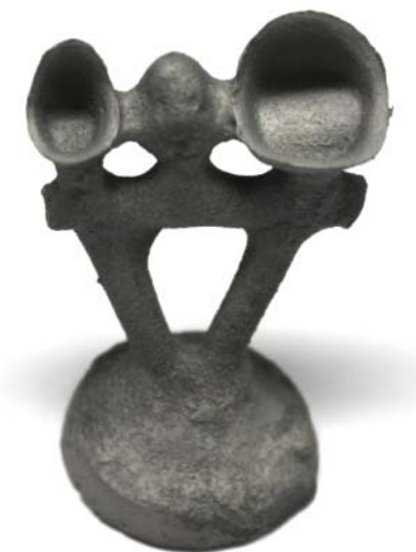
Fig. 8. Casting made construction with casting channels and feeders
