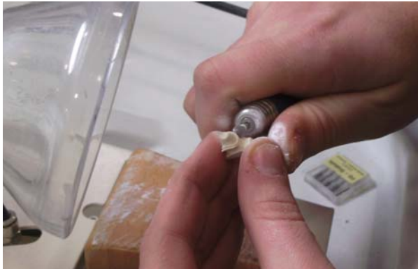
Fig. 3. Additional preparation of plaster model for optical scanning
