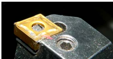
Fig. 21. The wear of cutting insert Sumitomo
