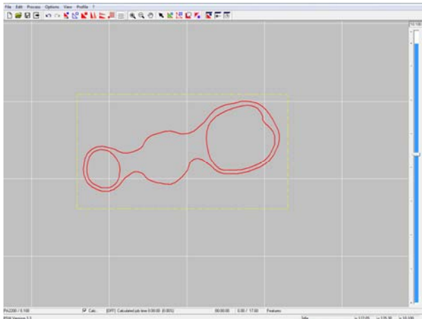
Fig. 7. Sliced three-dimensional model in layers positioned on work tray
