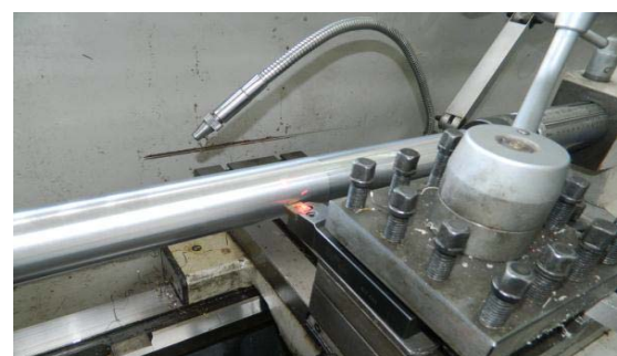
Fig. 8. The turning process of stainless steel material
