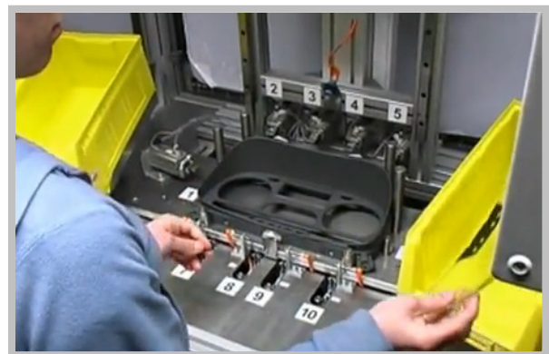
Fig. 4. View at manual assembly workplace, equipped with sensors to control assembly process [1]
