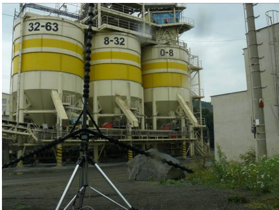
Fig. 12. Installed Acoustic Camera by tanks in stone quarry.
