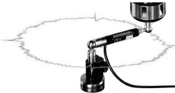
Fig. 2 Detail of the system Renishaw Ballbar QC10
