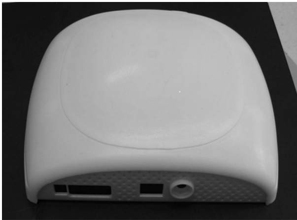
Fig.6. Finished prototype made by combination of SRM (cover) and PolyJet™ (back plate) rapid manufacturing technologies
