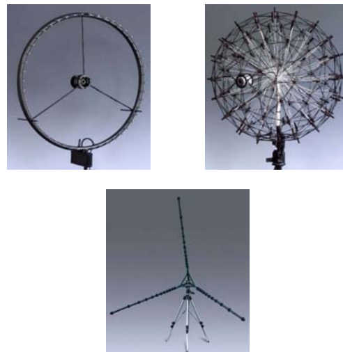
Fig. 1. Microphone Arrays (Ring, Star and Sphere)
