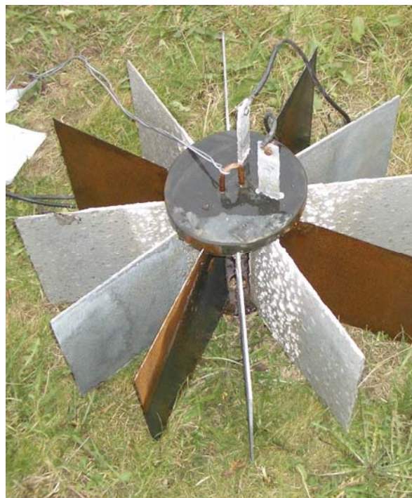
Fig. 2 Star electrode construction for water waste cleaning of the blast radius of SO
