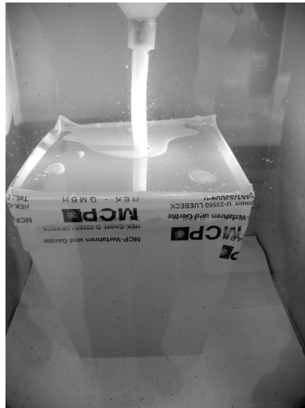
Fig. 3. Vacuum casting into SRM mould.
