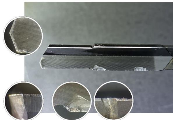
**Fig. 6a** Coolant Pressure Increased by 5 Bar to 55 Bar for Cooling, Lubrication, and Chip Flushing: Damage to the new (factory-reground) drill.
