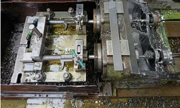
**Fig. 1** Tool testing in the deep drilling process: Machine in operation.
