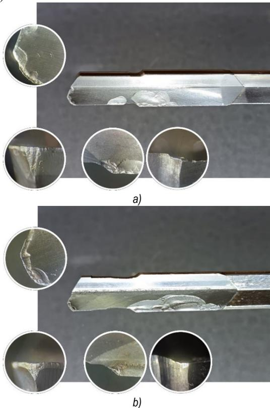
**Fig. 5** Coolant Pressure at 50 bar for Chip Flushing: a) Damage to the new (factory-reground) drill, and b) Damage to the reground drill.
