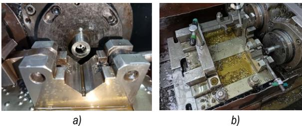
**Fig. 2** Tools and Fixtures for Workpiece Clamping: a) Bushing with a gun drill for initial drill guidance, and b) Prisms for workpiece clamping and centering
