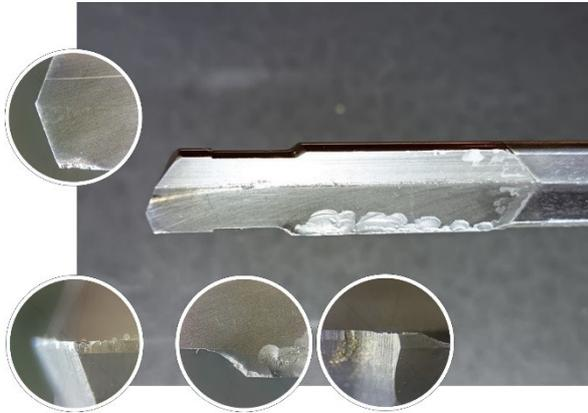
**Fig. 6b** Coolant Pressure Increased by 5 Bar to 55 Bar for Cooling, Lubrication, and Chip Flushing: Damage to the reground drill.
