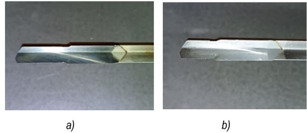
**Fig. 3** Condition of Drills Before Testing: a) Factory-Reground Drill, and b) Subsequently Reground Drill.
