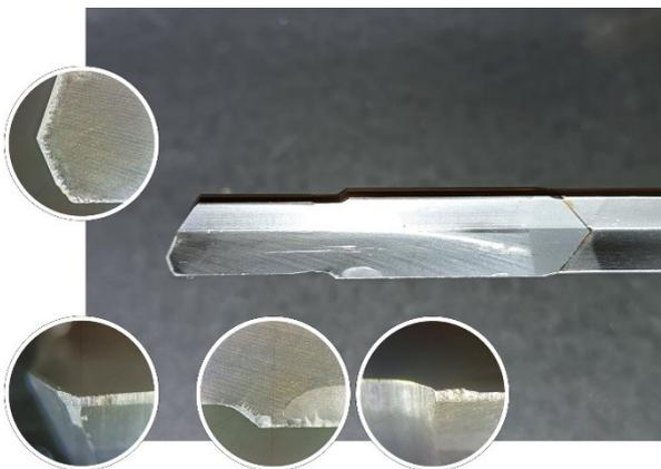
**Fig. 7a** Coolant Pressure Increased by 5 Bar to 60 Bar for Cooling, Lubrication, and Chip Flushing: Damage to the new (factory-reground) drill.
