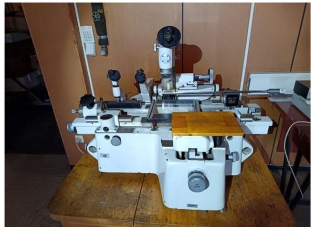
**Fig. 4** Measurement of wear bands using the universal measuring microscope UIM-21.
