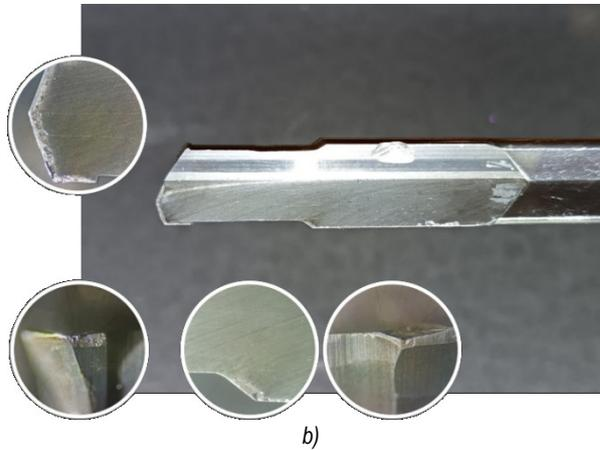
**Fig. 7b** Coolant Pressure Increased by 5 Bar to 60 Bar for Cooling, Lubrication, and Chip Flushing: Damage to the reground drill.
