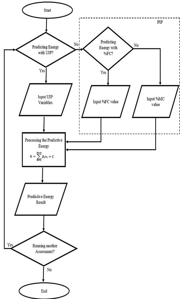
**Fig. 5** Flowchart of the computer program development.
