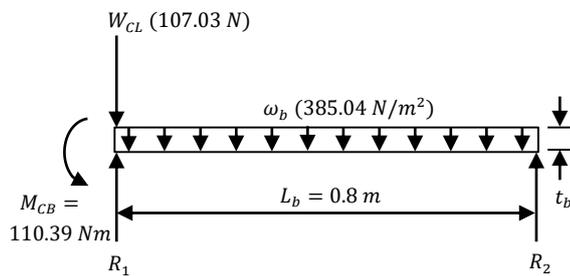
Fig. 3 Free body diagram of the base.
