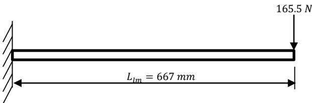
**Fig. 2 Free body diagram of the first loom as a cantilever.**
