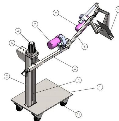
Fig. 1 Isometric view of the drainage clearing machine.
