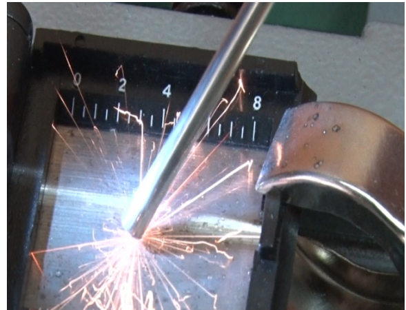
Fig. 2. Effect of a short circuit between aluminum and steel
