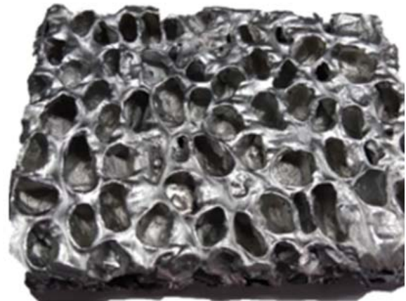
Fig. 1. Front view of the closed cell metallic foam with aluminum as a based material prepared by using ALUHAB Technology
