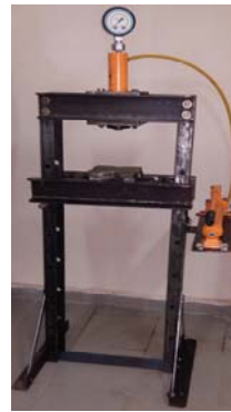
Fig. 2. Pictorial view of the 10 tons hydraulic press
