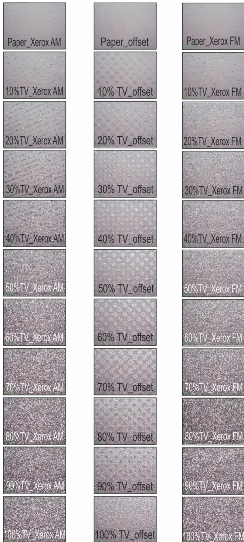
» Figure 5: Images of segment silver imprints enlarged 160 times (after experimental printing)
