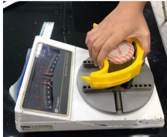
» Figure 2: Mechanical torque meter and grip posture of force measurement
