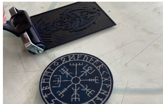
» Figure 8: Ink application on the surface of the printing plates. Produced by the author
