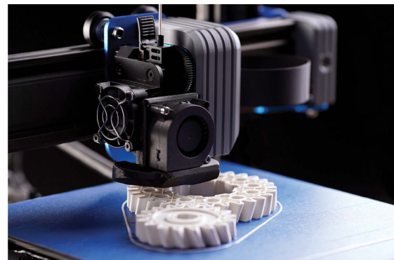
» Figure 2: Image of a printing FDM-type 3D printer (HLHRapid, 2023)
