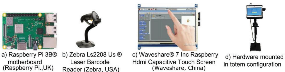
Figure 4. RAST 4.0 hardware. Source: Authors own work.
