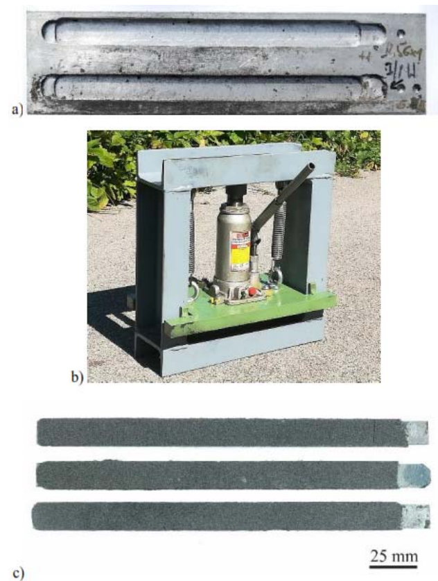
Fig. 1 a) Aluminum model for casting of rectangular coatings; b) Hydraulic press for coating compression; c) Coated electrode of rectangular core cross-section 12.56×1 mm 2
