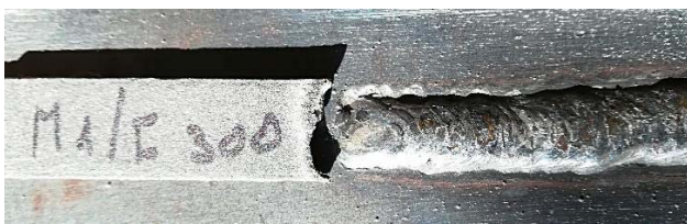
Fig. 2 The rectangular electrode after welding and the weld. The electrode burned evenly. The slag was easy to remove, little spatter.
