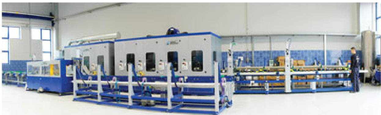
Fig. 3. The entire machine for grinding and polishing of circular stainless steel tubes
