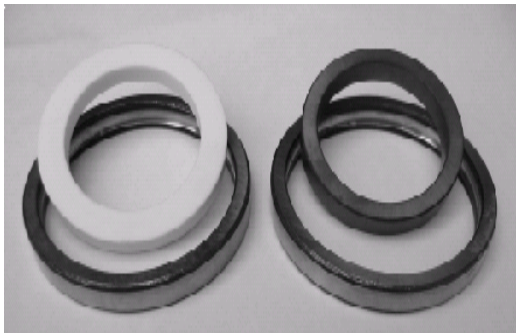
Fig.2 SiSiC and Al 2 O 3 rings
