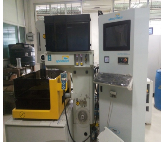
Fig. 1. Experimental setup of WEDM process
