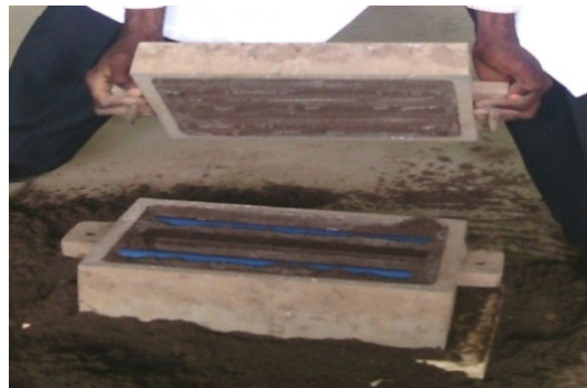
(g) Opening to remove patterns
