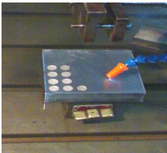
Fig. 2. Hot die steel H11 during Machining
