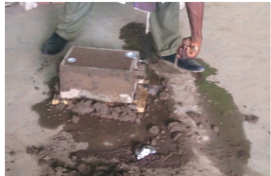
(b) Mold Filled with Molten metal.
