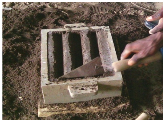
(h) Dressing and gating of the mould
