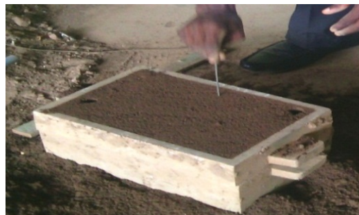
(f) Venting of the mould.
