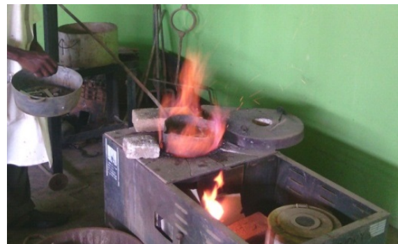
(b) Charging of scraps for melting.
