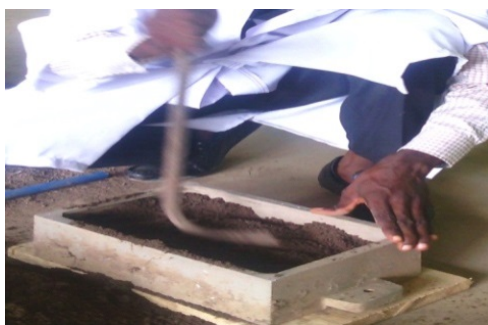
(b) Filling and ramming of mould
