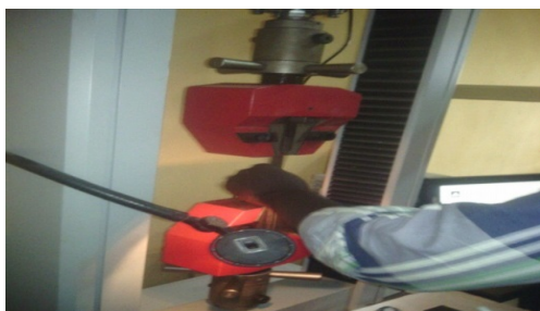
5.a) Fixing of a specimen unto the tensile testing machine
