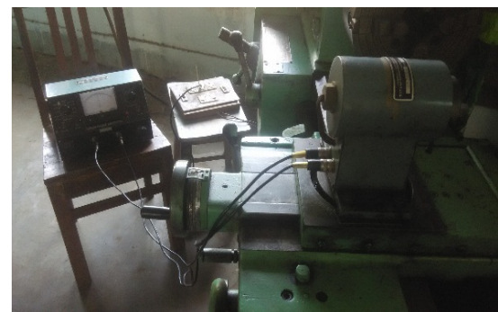
Fig. 2. Machining on lathe with tool dynamometers
