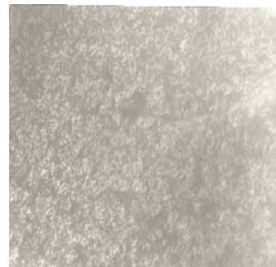
Plate 1. Photomicrograph of cast aluminium alloy using Idah silica sand (X100)
