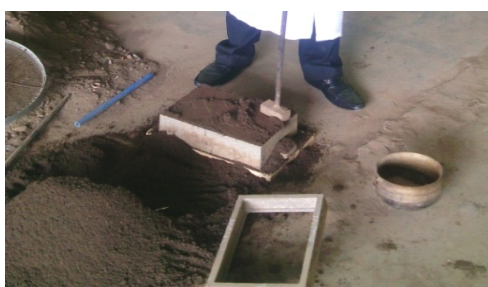
(c) Top filling of the drag
