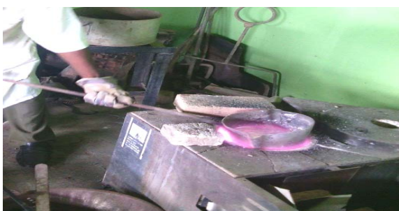
(d) Removing of molten metal from furnace Plates 2. Melting of Metal
