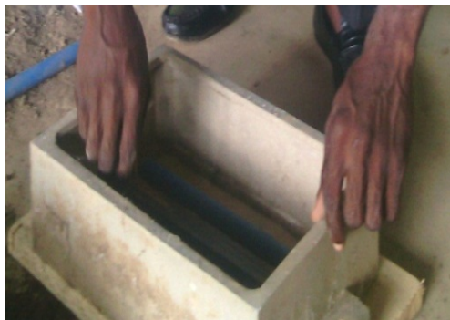
(a) Placing of pattern on the moulding board
