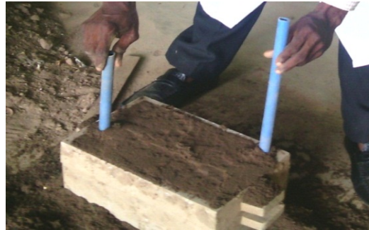
(e) Removing of runners & riser
