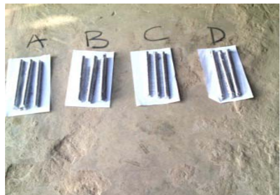
(e) Fettled casts. Plates 3. Casting of mould.
