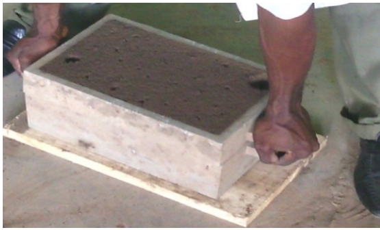
(i) Covering of the mould ready for casting Plate 1. Preparation of mould for casting aluminum
