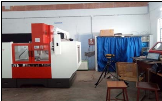
Fig. 1. Three axis CNC vertical milling machine with Laser Doppler Vibrometer (LDV)
