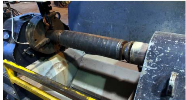
Fig. 4. Roller with hardfacing layer before machining process
