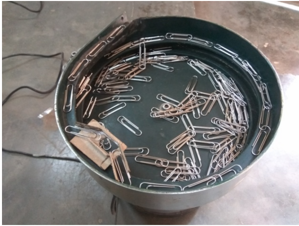
Fig. 2. Vibratory bowl feeder with modified path
