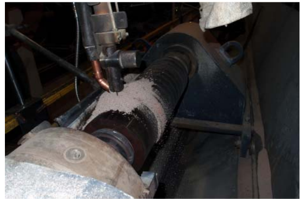
Fig. 3. Cladding layer formation process
