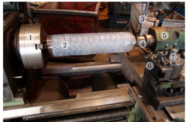
Fig. 5. Experimental configuration (1 – 3 jaws chuck, 2 – workpiece, 3 – coolant supply, 4 – tailstock quill, 5 – tailstock assembly, 6 – cutting tool, 7 – tool post)
