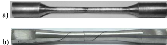
Fig. 3. Specimens after deformation: a) uni-axial tension, b) torsion
