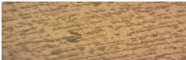
Fig. 6(c) Wet weld (200°C PWHT) X200
