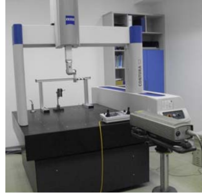
Fig. 4. Numerically controlled measuring machine with mounted LMS
