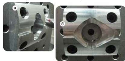
Fig.8. Stock (a), and machined contour (b), in machining test
