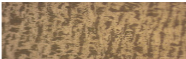
Fig. 6(e) Wet weld (400°C PWHT) X200
