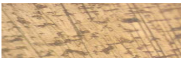
Fig. 6(f) Dry weld (400°C PWHT) X200
