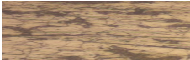
Fig. 6(a) Wet weld (as-weld) X200
