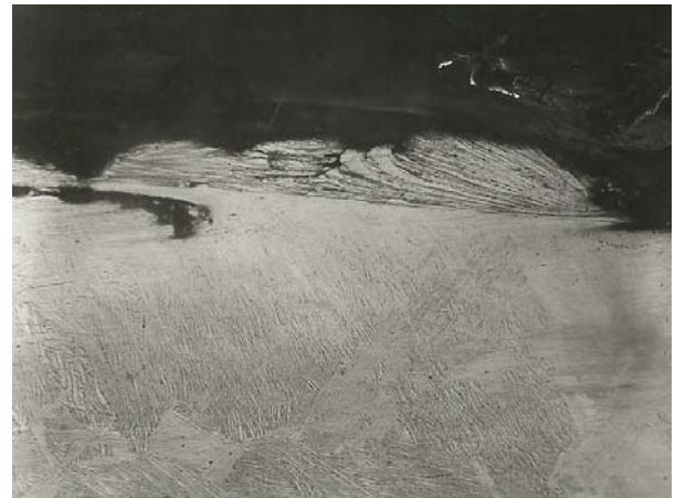
Fig. 11. Metallographic cut of chip creation during grinding titanium alloy VT 6 with Al_2O_3 tool
