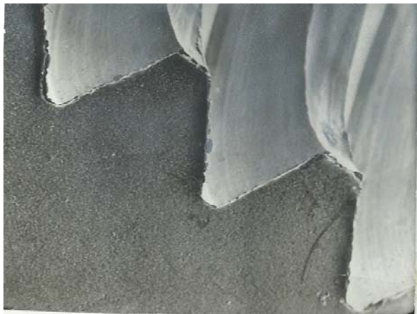
Fig. 10. View of thread made by a tap oscillated by ultrasound
