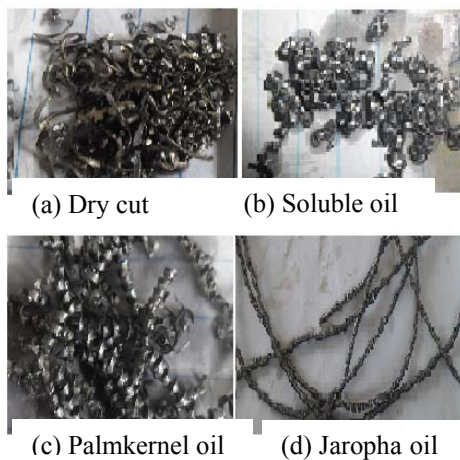
Fig. 7. Chips formation at spindle speed of 190 rpm
