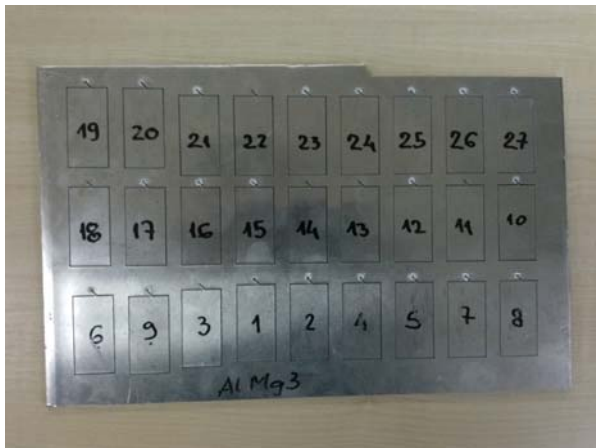
Fig. 1. Plate with specimens obtained after laser cutting,
