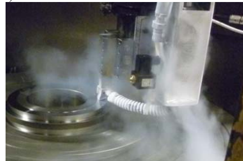
Fig. 25. Gas leakage of nitrogen a) via safety valve of the tank b) during cutting via phase separator
