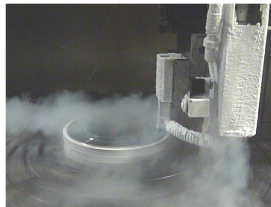
Fig. 26. Cooling of the workpiece during flood cryogenic cooling
