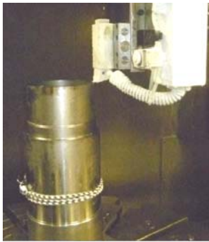
Fig. 22. Turning of Ti-6Al-4V with a coated carbide insert with cryogenic cooling [17]
