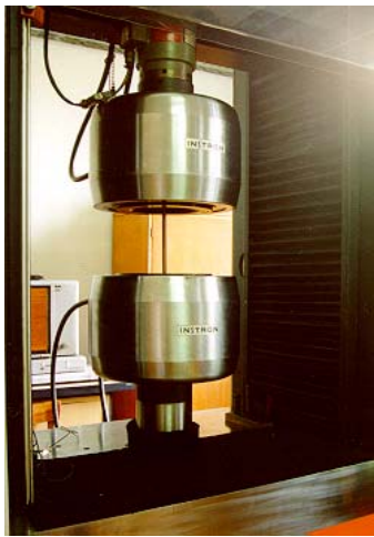
Fig. 2 Universal static-dynamic testing machine INSTRON 1255.
