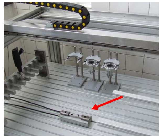
Fig. 4 Present status of pneumatic clamp in the flexible production cell
