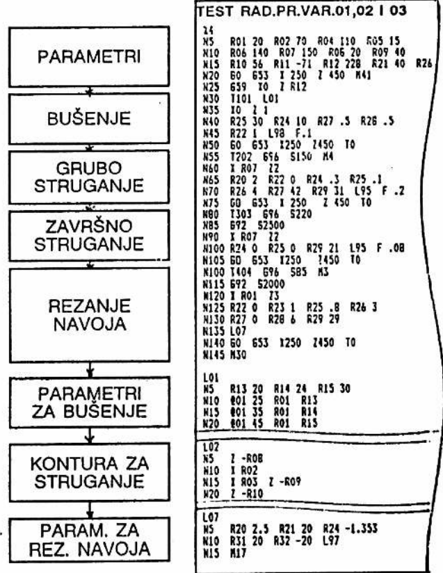
Sl.4 Upravljački programi pisani metodama pogonskog programiranja Fig. 4. NC part programs written by workshop programming methods
