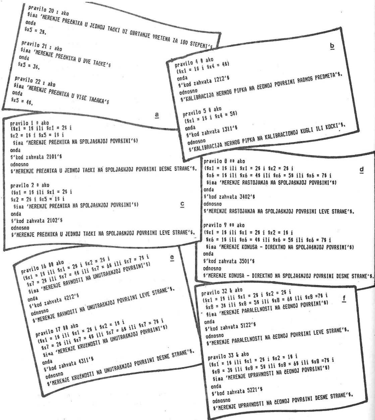
Slika 5. Deo pravila za definisanje klasifikacionog broja (a), merno-kontrolnih zahvata kalibracije mernog pipka (b), merenja prečnika (c), dužinska merenja (d), merenje odstupanja od oblika (e) i položaja (f) Figure 5. Part of the Rules for Defining of Classification Number (a), Measuring and Inspection Operations for Probes Calibration (b), Diameters Measuring (c), Length Measuring (d), Form Measuring (e) and Position Measuring (f)
