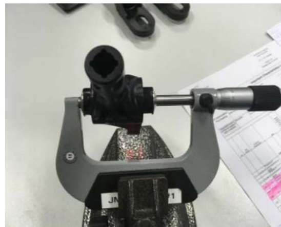
Fig. 2. Acquisition of measurement data for process capability analysis
