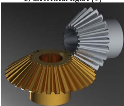
b) CAD model of our designed gear pair ( \Sigma=80^\circ )
