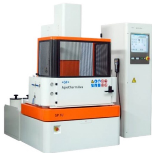
Fig. 2. EDM machine Agie Charmilles of the SP1-U type
