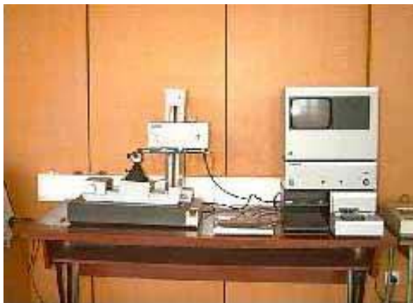
Fig. 1. Surface roughness measurement system Talysurf 6
