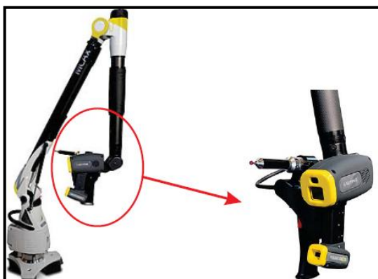
Fig. 3. MMDx100 laser scanner integrated with Nikon MCAx+2.0 measuring arm
