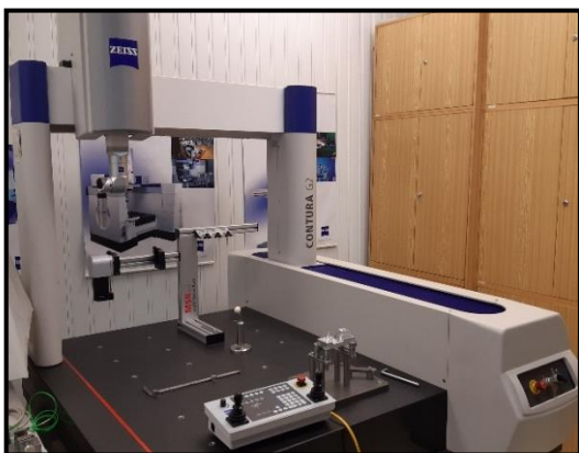
Fig. 2. Coordinate measuring machine Carl Zeiss Contura G2 RDS
