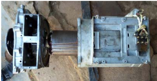
Fig. 8. Assembly of all the generator components
