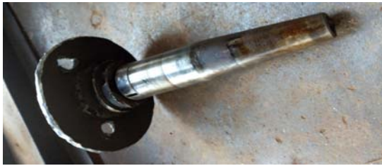
Fig. 7. Shaft geometry after turning operation
