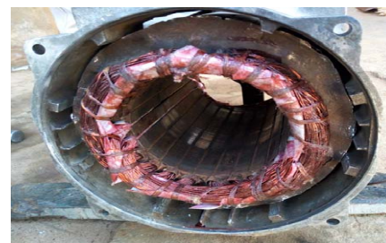
Fig. 4. The stator after rewinding and varnishing
