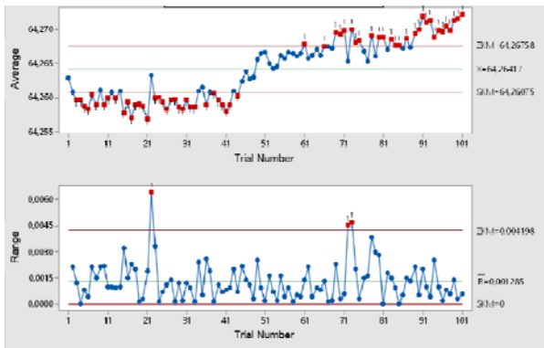
Fig. 6. X – R chart of measurements for diameter \phi 64.3 mm.
