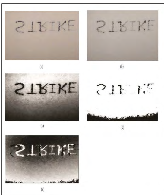
» Figure 11: (a) Original image (b) RGB to Gray Converted image (c) Histogram Equalized Image (d) Foreground Image (e) Detected Strikethrough Pixels
