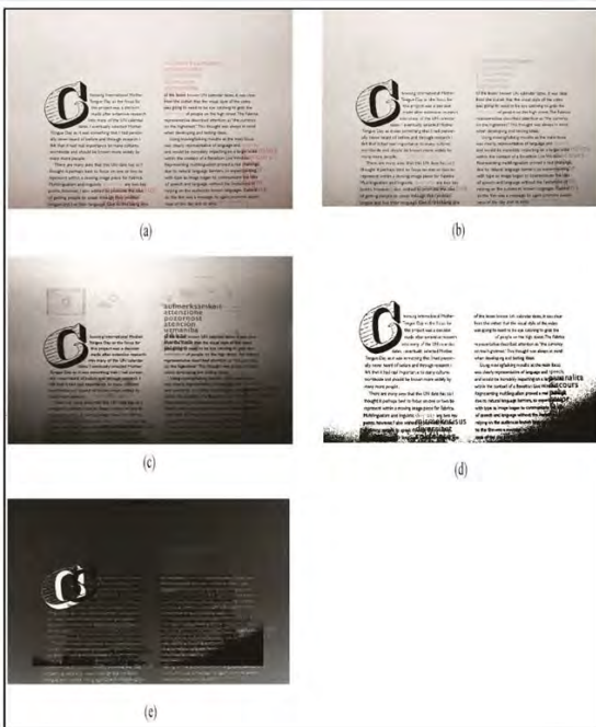
» Figure 6: (a) Original image (b) RGB to Gray Converted image (c) Histogram Equalized Image (d) Foreground Image (e) Detected Showthrough Pixels
