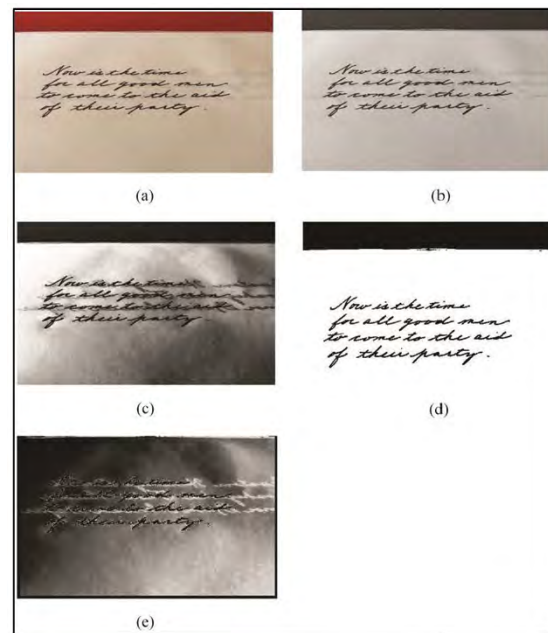
» Figure 4: (a) Original image (b) RGB to Gray Converted image (c) Histogram Equalized Image (d) Foreground Image (e) Detected Showthrough Pixels.
