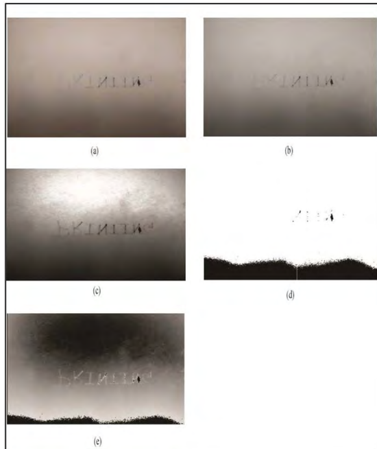
» Figure 8: (a) Original image (b) RGB to Gray Converted image (c) Histogram Equalized Image (d) Foreground Image (e) Detected Strikethrough Pixels
