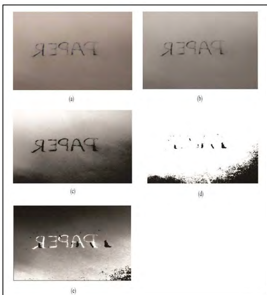
» Figure 10: (a) Original image (b) RGB to Gray Converted image (c) Histogram Equalized Image (d) Foreground Image (e) Detected Strikethrough Pixels
