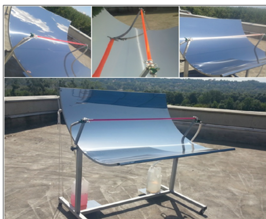
» Figure 2: Solar Parabolic reactor used for photocatalytic experiments
