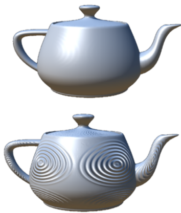
» Figure 2: Comparison of a teapot rendered using texture mapping (top) and bump mapping (bottom)
