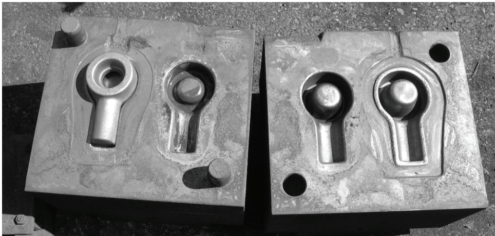
Figure 18 - Final shape of the forged joint socket
