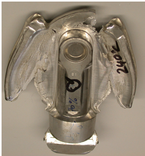
Figure 7 - Footprint of shock absorber head forged at 240°C from AZ80 alloy [14].
