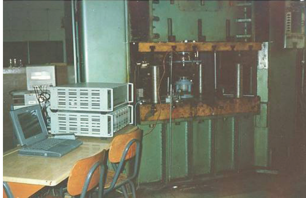
Fig. 4 - Hydraulic Press with Measuring Equipment
