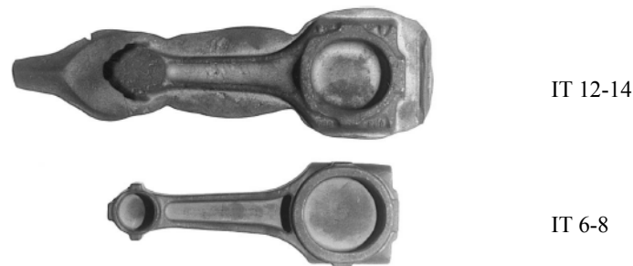
Figure 1 – Connected rod obtained by conventional and precision (flashless) forging [9]
