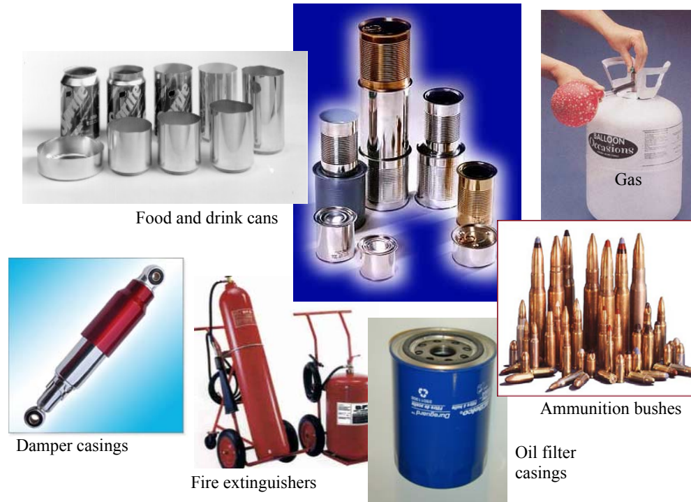
Figure 1 - Examples of some parts manufactured by ironing.
