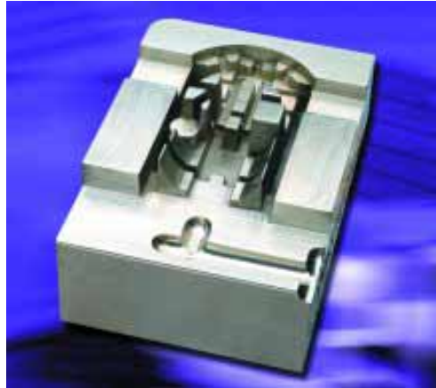
Figure 5. The tool gotten by SLS process [18]
