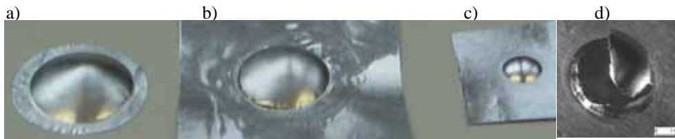
Fig. 8: Stretch-formed parts, produced with 50 CO 2 -laser pulses a) \varnothing 12.3 mm; height 2.4 mm b) \varnothing 11 mm; height 1.9 mm c)/d) \varnothing 4 mm; height 0.84mm
