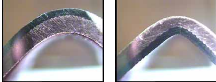
Picture 5. Tapered and increased thickness of layers of materials at banding of two layer composite C4580-Cu99,9 with radius punch r_i=2\text{mm}
