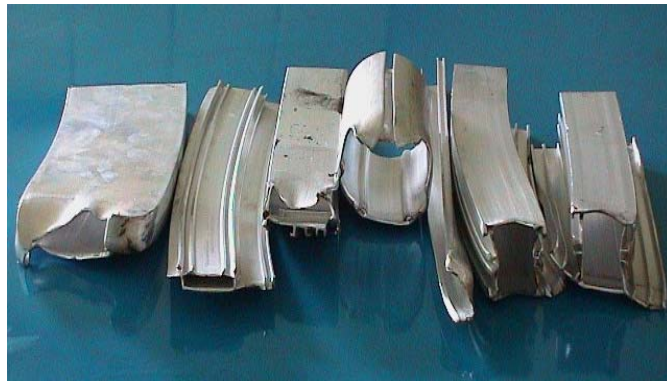
Fig.1.2 Defects on extruded profiles
