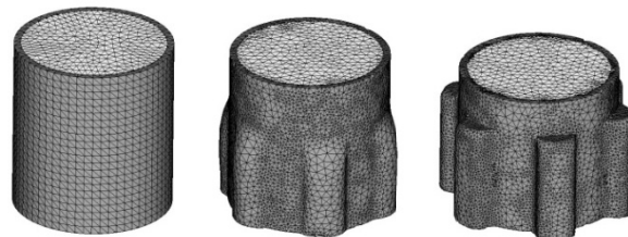
Fig.10 – Workpiece at the beginning, during and at the end of simulation [9]
