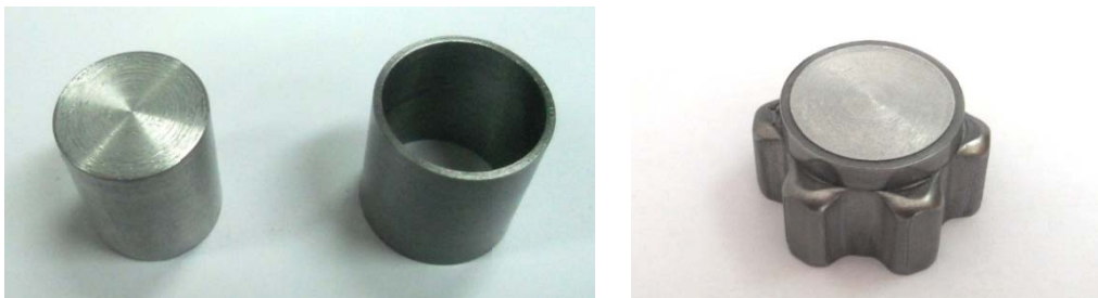
Fig.11 – Disassembled Al/Steel billet (left) and workpiece after radial extrusion (right)
