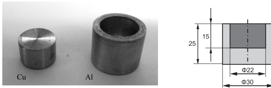
Fig.6 - Photograph of aluminum sleeve and copper core and dimensions of composed billet
